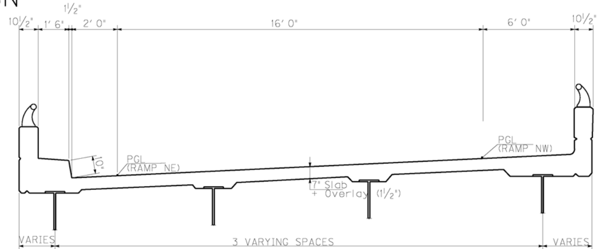
TYPICAL CROSS SECTION SPANS 9-12
